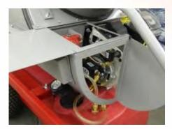
The Optional Heat Recovery System (HRS) from Frost Fighter reduces nuisance service calls in applications affected by severe cold, precipitation and condensation.
